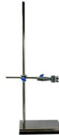
12. Boss, clamp and stand Attaches to and holds other pieces of equipment
